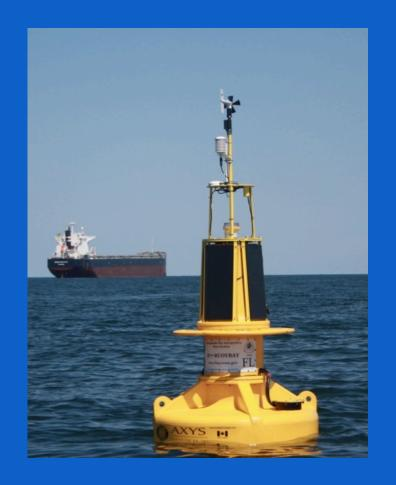
Technologies TRIAXYS wave sensors centrally mounted in the buoy hull. The CBIBS buoys represent the only real-time wave measurements within the Chesapeake Bay. Results of a comparison between CBIBS buoymounted currents and waves and independent coincident data are presented in Wilson and Siegel, MTS/ONR Buoy Workshop, 2011.
